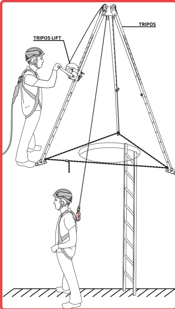
TRIPOS and two COBRA LIFT, two users, with risk of falling from a height
