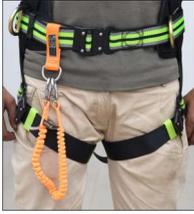
Once the anchor point and the lanyard are selected, the connections can be made using aluminium connector, TS 90 001 07.
